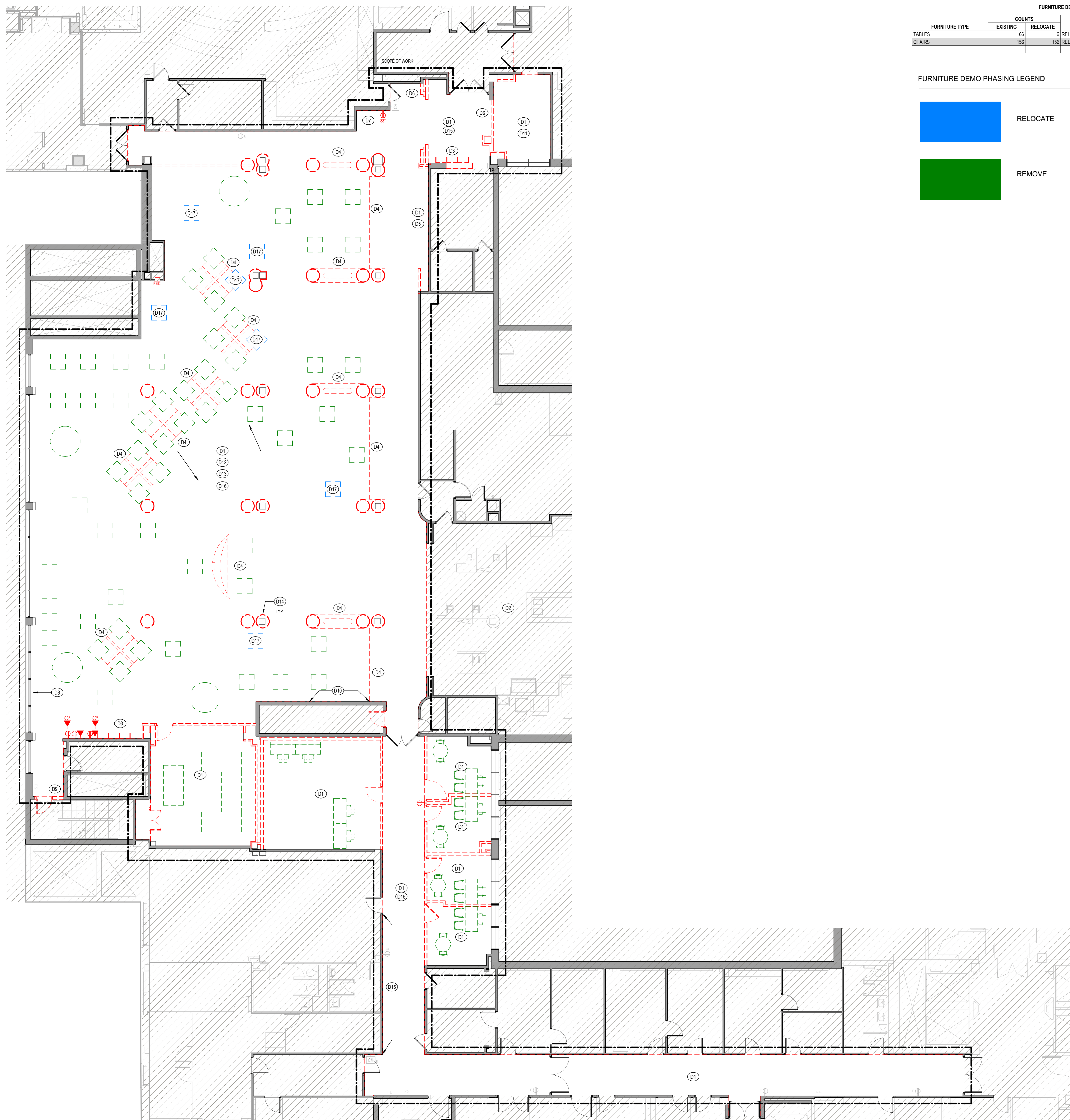
1 SECOND FLOOR DEMOLITION PLAN 1/8" = 1'-0"
